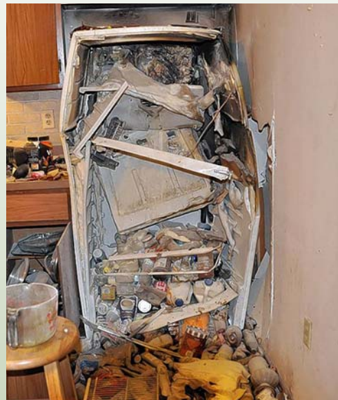
Refrigerator exploded due to accumulated flammable vapors.
