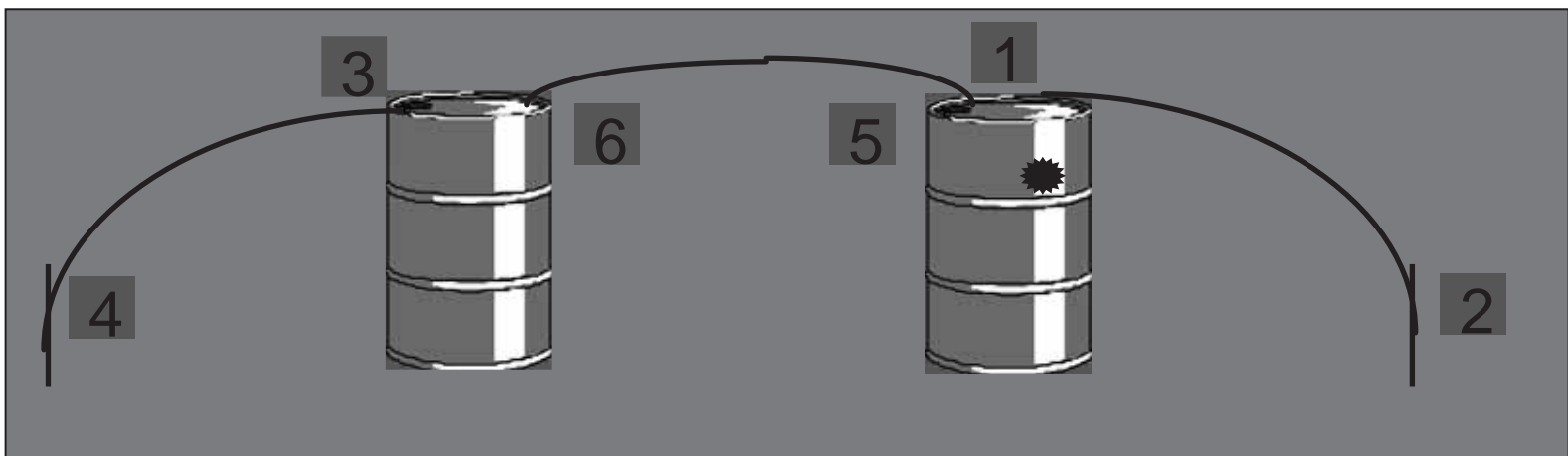
Figure 17.1: Grounding and bonding procedure
