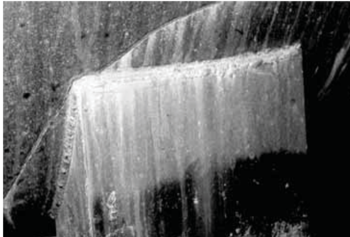
Figure 18.2 Cracks in the Inner Tank Shell
