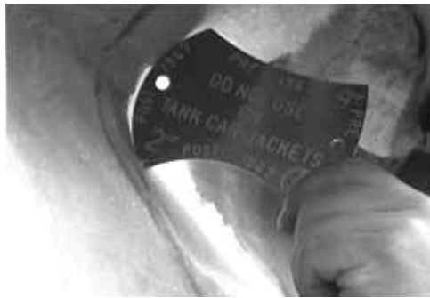
Figure 18.3 A dent gauge is used to measure the radius of a dent
