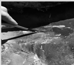
Caused by contact with other metal
