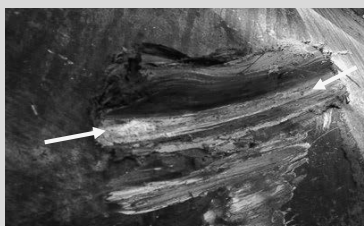
Associated with wheel and rail burns
